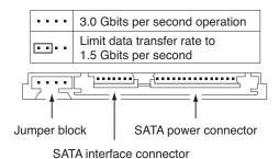
Figure 3. Serial ATA connectors
